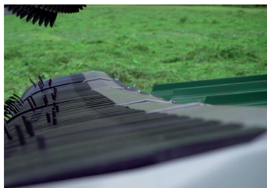
Instead of the straight line contact the flexible pick-up contacts the ground in a curved line for optimal ground hugging.
