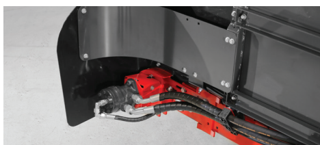
The direction and speed of the conveyor belt are simply carried out by a hydraulic motor.
