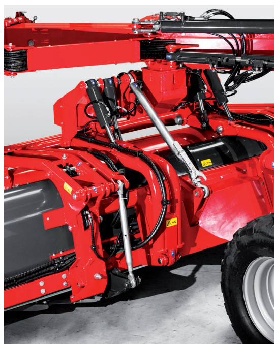
The pick-up unit on the flexible frame with hydro-pneumatic suspension system ensures excellent responsiveness to the uneven terrain.
